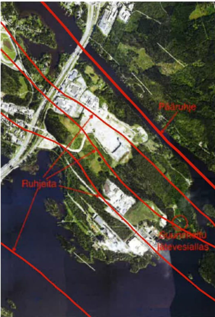
Image 3. Map of the soil fractures in Sorsasalo (source GTK). The locations of the fractures have been highlighted in red.
